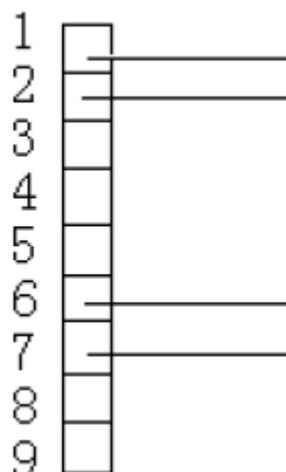
Note: Please do not connect any wire on Pin3 and Pin4 if com1 is no use, if the two use different power supply, please make sure the two use the same GND (join the two`s GND together)
