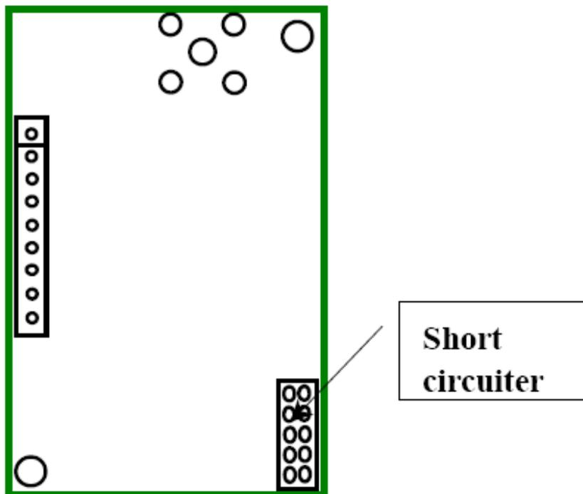
There is one group of 5-bit short-circuiter wire (JP2) on the bottom right corner of HR-1102, defined as A、B、C、D、E respectively. Assuming the open circuit of jumper wire (without short circuiter) is mode 1 and short-circuit of jumper wire (with short-circuiter) is mode 0.
