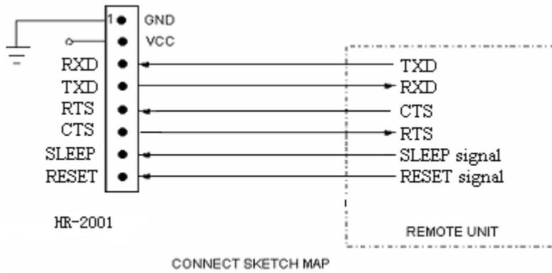
**Picture 1: Connection sketch between HR-2001 and terminal equipment**
