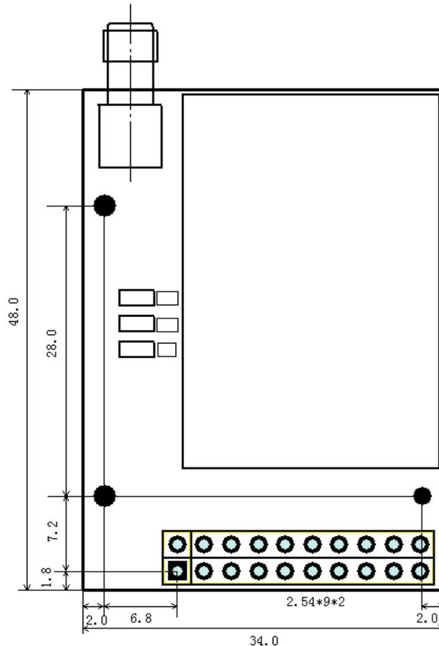
Picture 2 Structure dimension of HR-2001 V1.1
