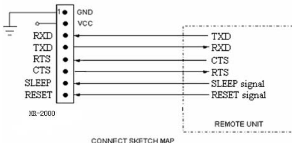
Picture 1: Connection sketch between HR-2000 and terminal equipment
