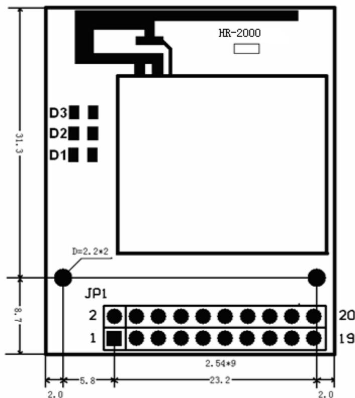
Picture 2 Structure dimension of HR-2000 V1.2
