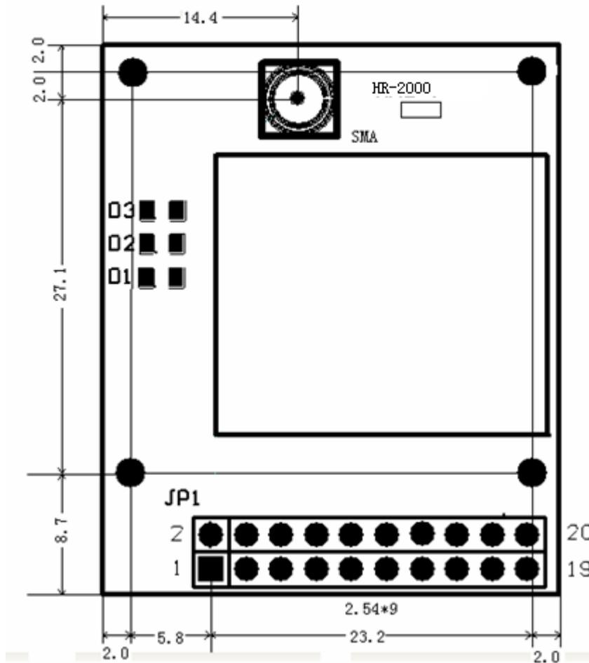
Picture 3 Structure dimension of HR-2000 V1.3
